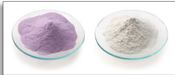
Potassium bicarbonate or “Purple-K Powder” (left) and sodium bicarbonate dry-chemical agents are displayed. Photo courtesy of the Fire Equipment Manufacturer's Equipment Association.
