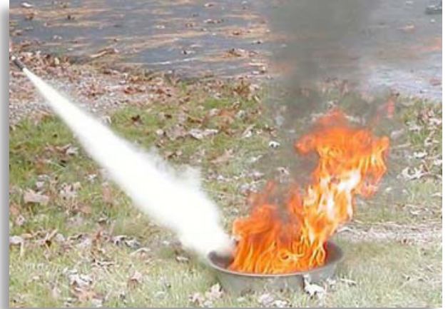
The streaming clean agent fire extinguisher will leave no residue after the fire is suppressed.
