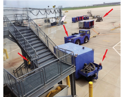
Airport Ramp Area. Arrows Indicate Extinguishers.
