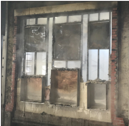
Photo B: Test structure for UL-1479
