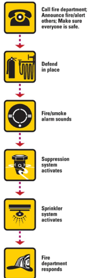
**extinguishers. They can extinguish fires during the incipient stage before they are large enough to trigger a sprinkler or other suppression system. This helps to protect against property damage and the buildup of dangerous smoke."**
