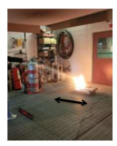
Figure 11: Participant using a sweeping motion to deploy agent on BullEx ITS
