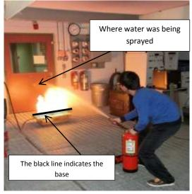
Figure 9: Participant aiming above the base of the BullEx ITS
